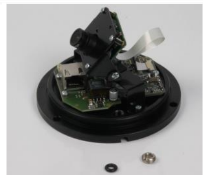
Screw off the cable fixer ring
