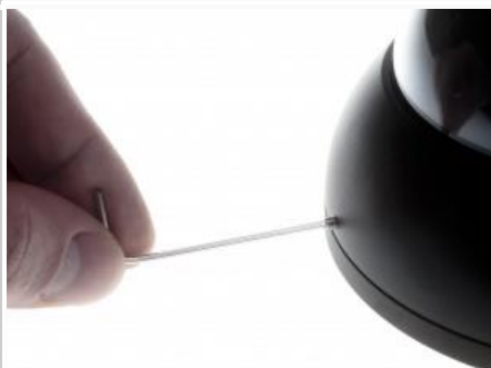
Screw off counter-clockwise the two screws
